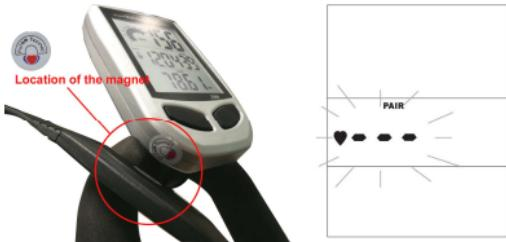
If the Heart Rate value is displayed on LCD, it means that the pair stage is successfully completed.
